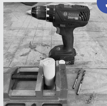
Drill a 40mm deep hole on both ends using a 6mm drill bit
