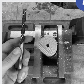
Drill a 15mm deep hole on both ends using an 8mm drill bit
