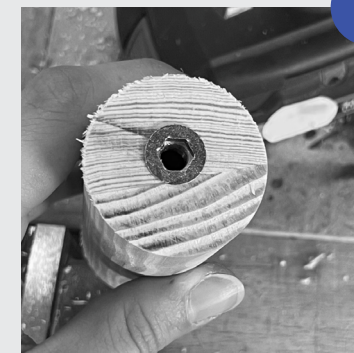
Screw insert nut into piece on both ends
